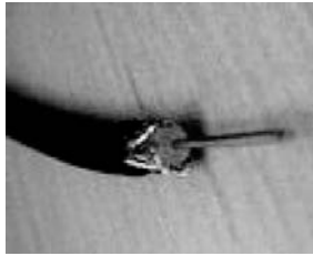
Figure 12: RG-8 coaxial cable.
